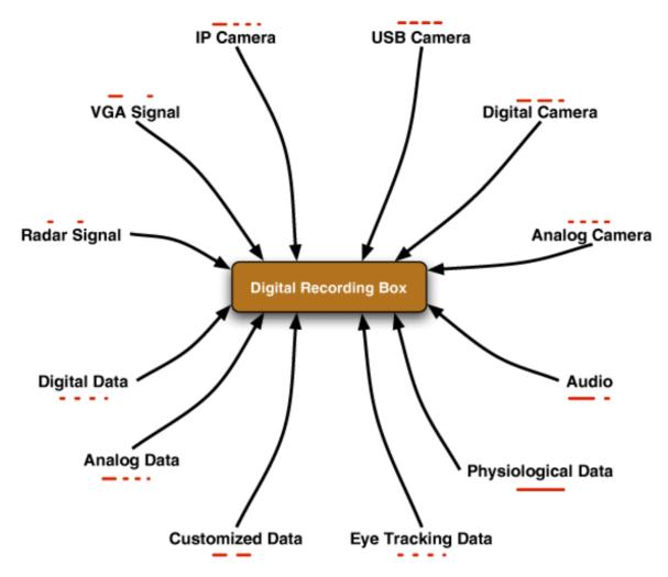
During the recording, all signals with their different timing, are recorded and synchronized in separate files. Of course it is also possible to assign for example the audio to a certain video stream and save the audio stream in this video file.
